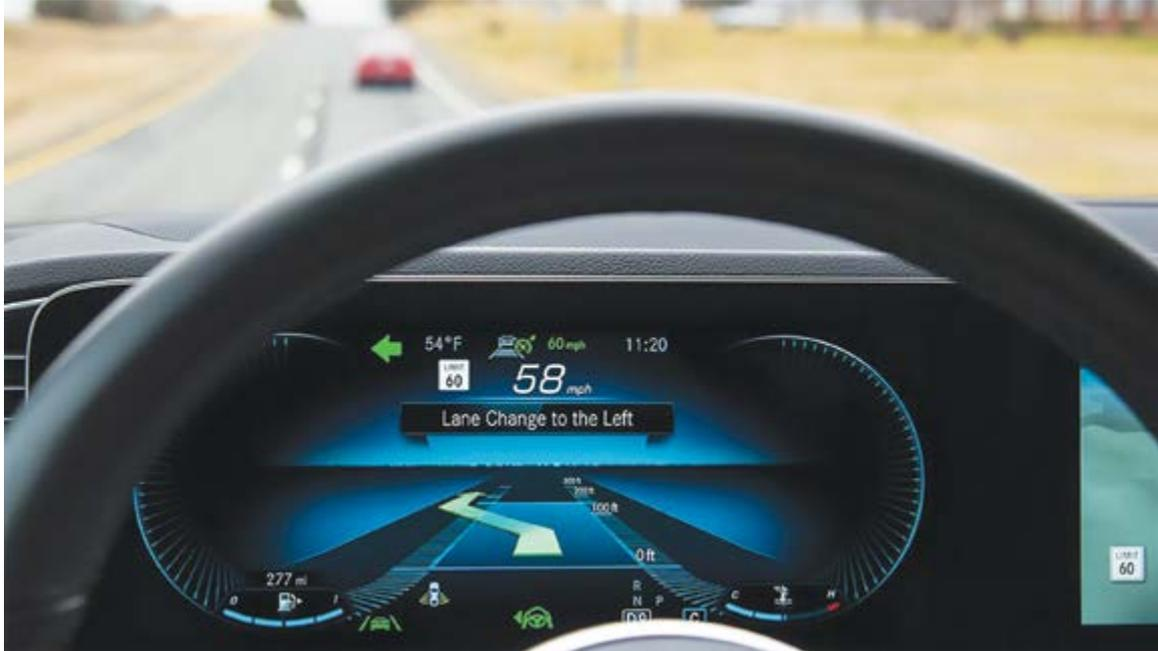
Several Level 2 systems, such as the one in this Mercedes-Benz GLE-Class, can already execute lane changes automatically, but IIHS researchers recommend against enabling that feature.
